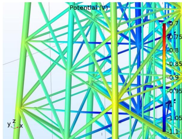
BEM modeling results for potential distribution (V vs Ag/AgCl)
