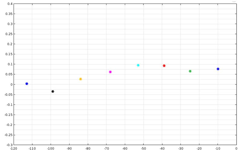
Potential (V vs Zn) vs elevation (m) predicted for reference electrodes of TSRE
