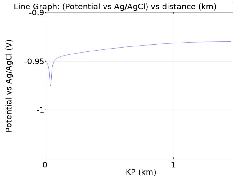
potential along the pipeline (note: only half pipeline shown)
