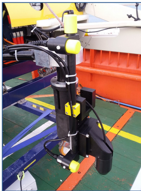
Fig. 6 – Subsea CP inspection system mounted on ROV
