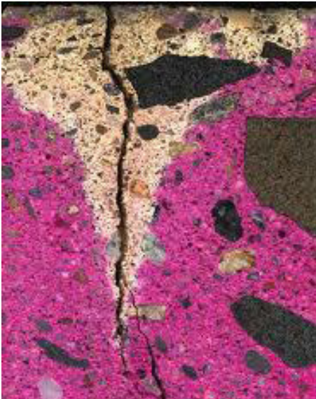
Carbonation test of concrete with phenolphthalein
