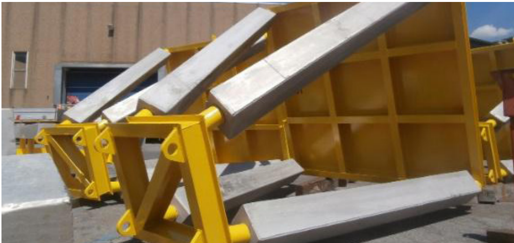
Anode pods with aluminium alloy – 300 kg anodes
