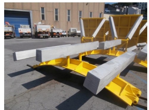
Segment of clamp with galvanic anodes (monopiles, single point moorings, etc)
